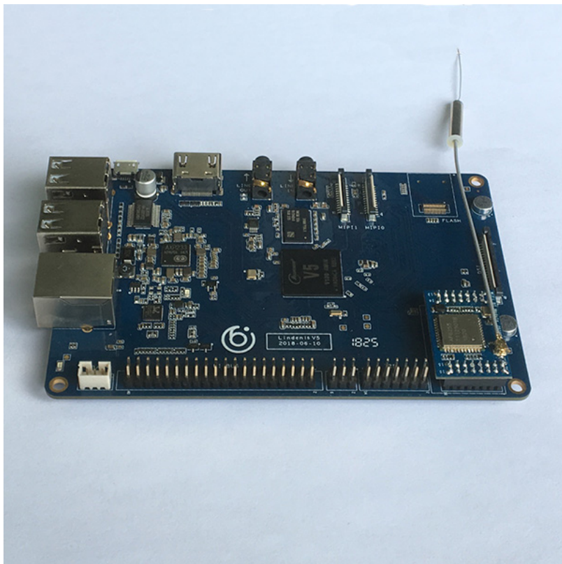
Figure 5: Linden V5 with Wi-Fi/BT module installed. Please match the pins when installing.
